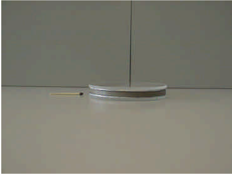
Fig. 8: The completed plate capacitor ( without connecting cables), compare size with match on left side
