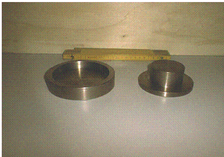
Fig. 2: Pressing tool, left of lower part, right of upper part
