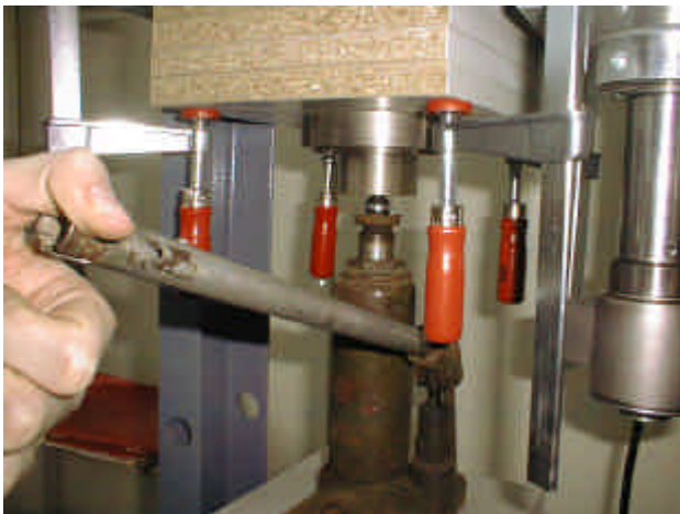
Fig. 4: Pressing the heated up Duracap material
