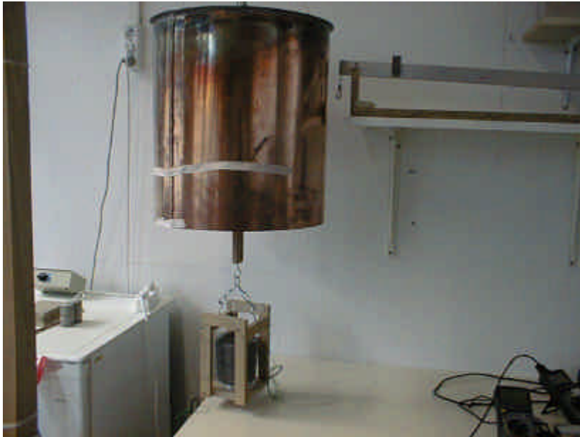
Fig. 12: Adjusting the copper cylinder, the wire wrap lines are not installed, see group of lines at right rear at hardwood frame.
