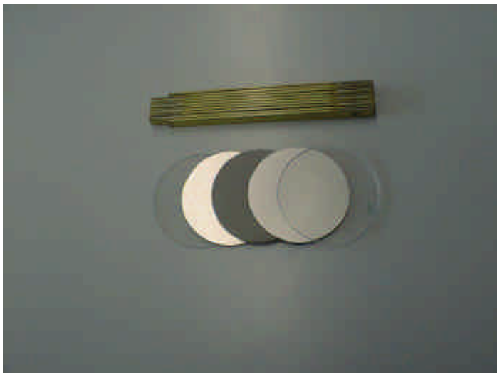
Fig. 7: Single components of the plate capacitor in exact order
