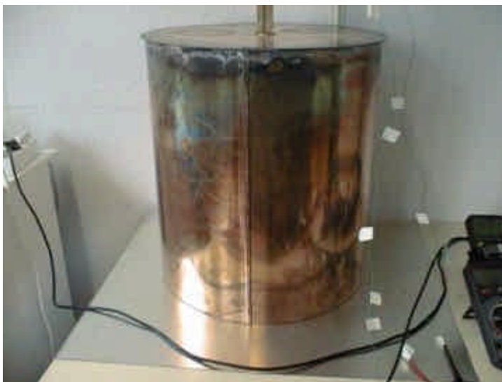
Fig. 14: Assembling the Faraday cage. The copper cylinder is placed on a grounded steel plate sealed with Cu foil .See picture above. The Hardwood bar is plugged through with glued on wire wrap lines. On the right of the copper cylinder are the wire lines, leading to measuring instrument and generator. On the wall suspension ( not in picture) the mechanical discharge takes place.( Lines are marked with several adhesive stripes for better identification )
