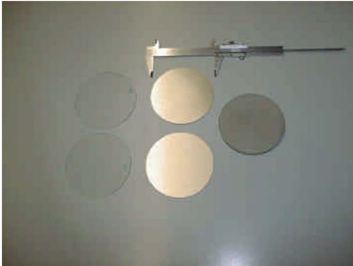
Fig. 6: Left: Plexiglas disks, center: Aluminum disks, right: Duracap disk
