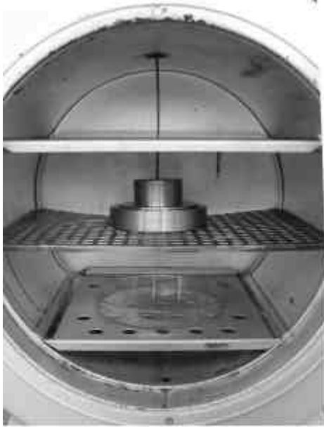
Fig. 3: Pressing tool in heating process together with Duracap granulates
