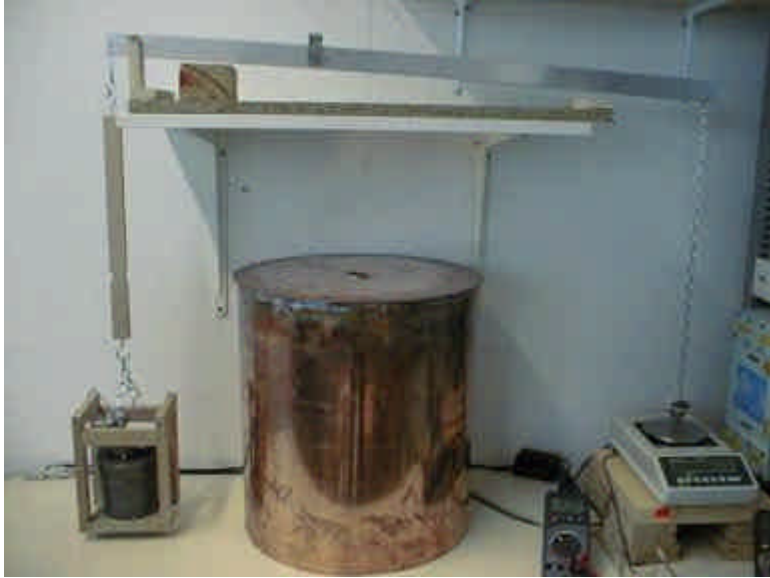
Fig. 10: Balance assembly with beam balance construction (photo), the copper cylinder in center of picture will be part of the Faraday cage
