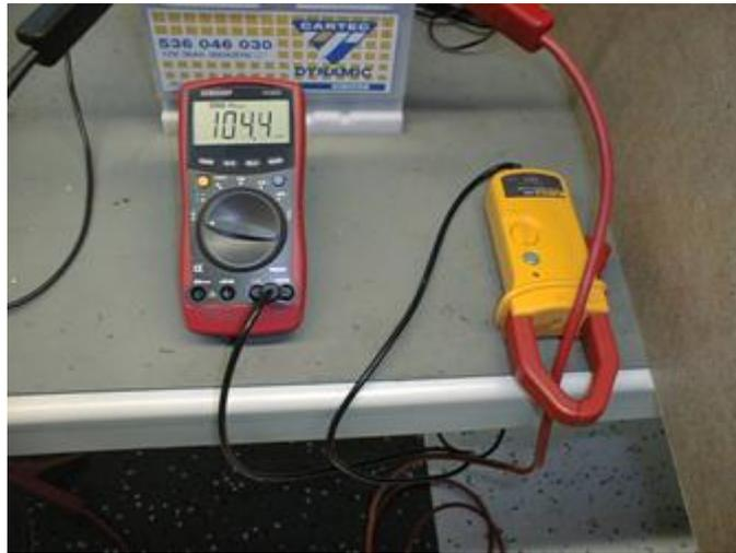
Fig. 20: Motor vehicle battery, clamp on ampere meter, coupled multimeter
