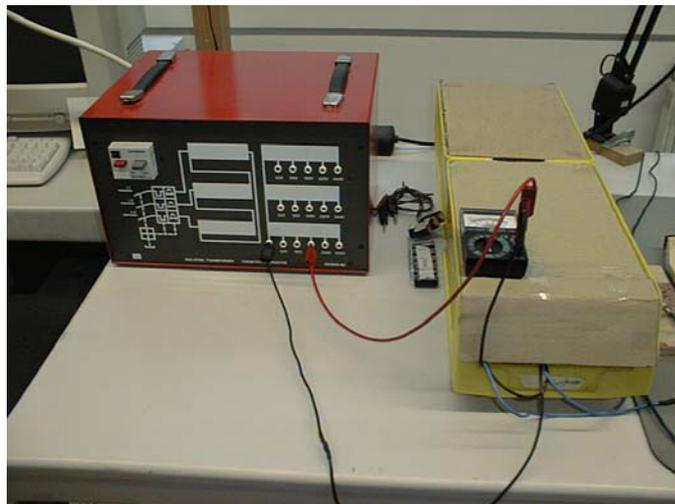
Abb. 4: Alternate current (left), by means of a electric rectifier (in the isolated housing right, together with the capacitor bank ) loading the condensers to a max. of 500 V.
