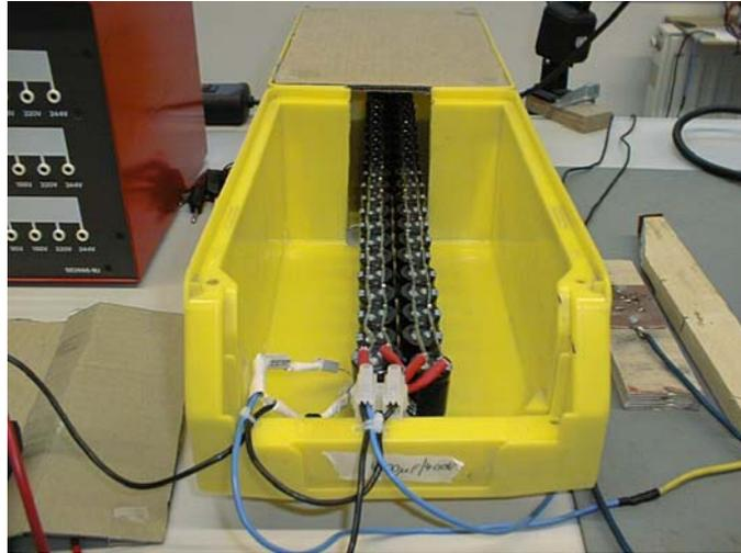
Abb. 3: Installation of capacitor bank into an isolated housing
