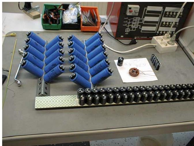
Fig. 2: Testing different capacitor combinations
