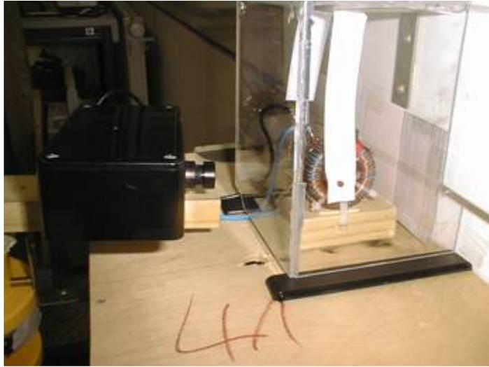
Fig. 8: A match is fastened to the paper strip, on the left camera to register movements of pin/match and paper stripe
