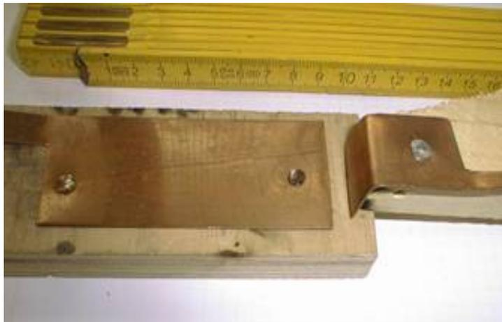
Fig. 5: Two new copper sheet contacts (power switch)
