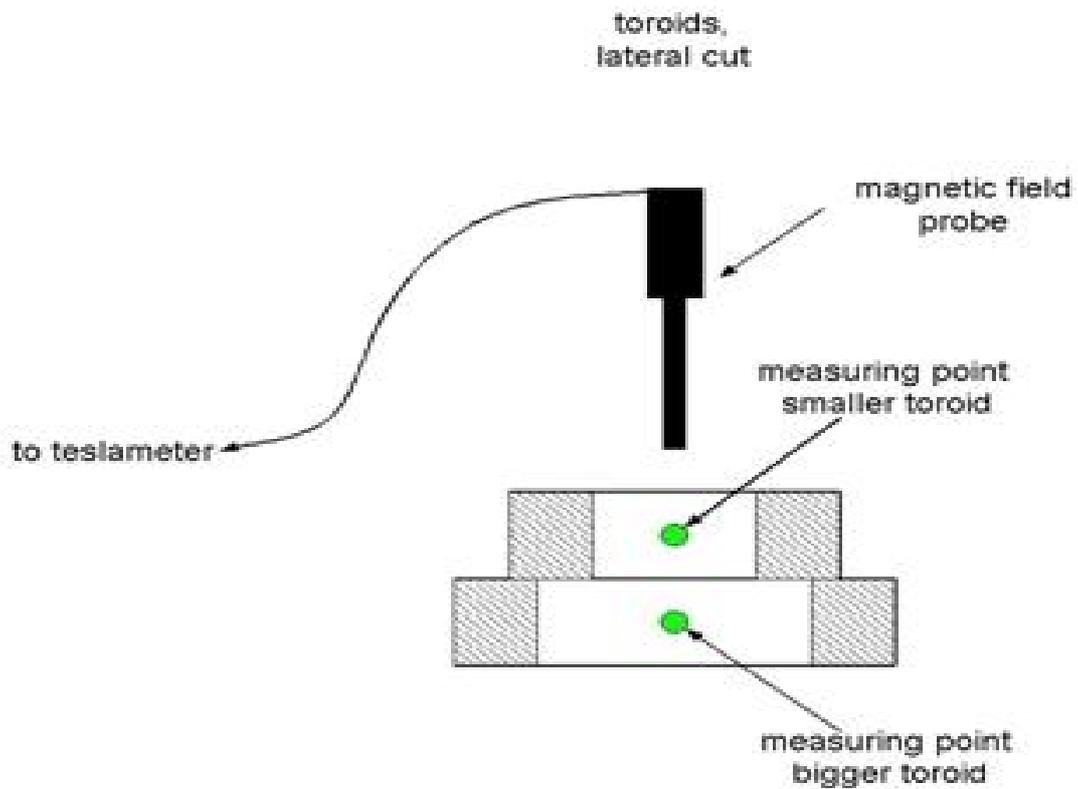
Fig. 21: Crosscut of the toroidal core combination and marking of two measuring points
