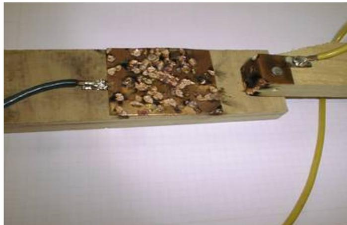
Fig. 6: Copper sheet contacts (power switch) after approx.50 times used as switch
