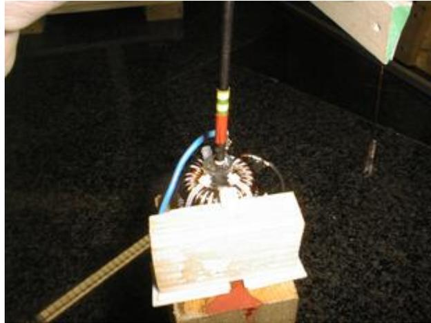
Fig. 22: Measurement of the leakage fields of the two toroidal coils
