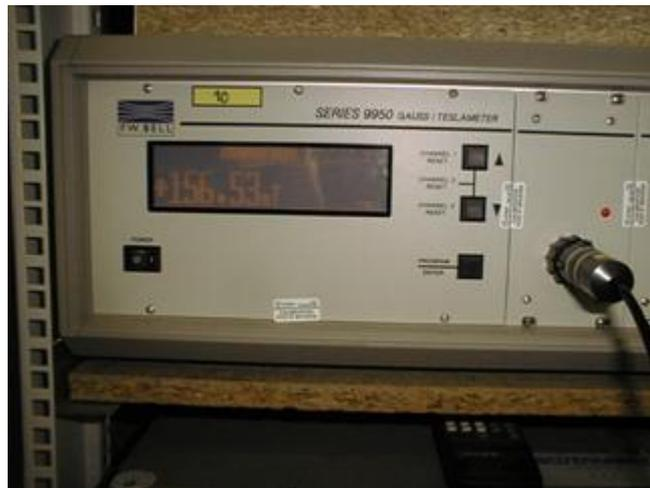
Fig. 19: Teslameter, F. W. Bell, Series 9950; in calibration phase of equipment
