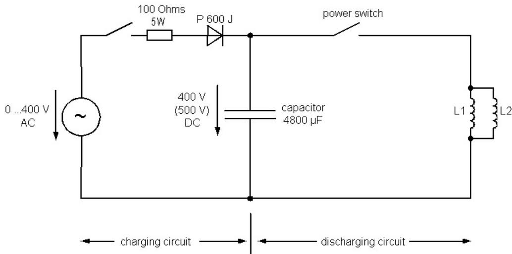
Fig. 7: Load and discharge current circle
