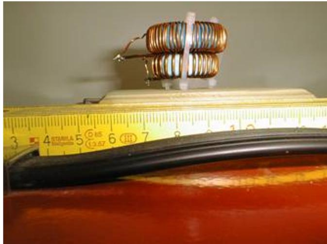
Fig.1: Toroidal coil combination L1, L2.
