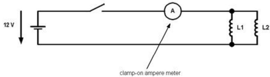
Fig. 18: Circuit diagram to determine the order of magnitude of the magnetic leakage fields
